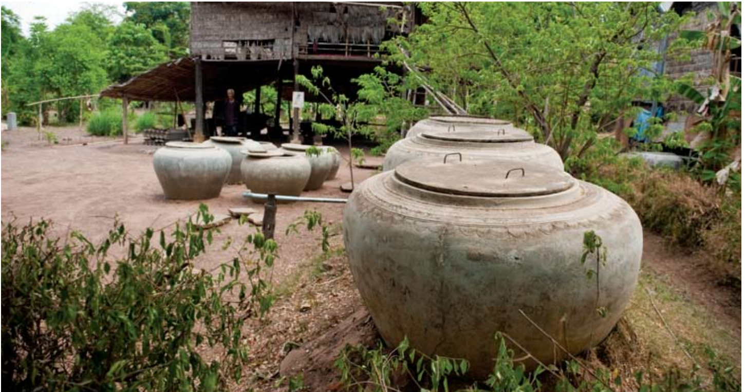
The use of cement jars for storage of rain water is very common in Cambodia.
